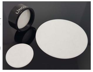
Our standard volume dispersion plates have a thickness of 0.5 mm with a diameter of 22.4 mm or 50.0 mm. On request, we offer further custom dimensions and UV resistant diffusor plates (applicable down to the DUV spectral range) for larger quantities.
