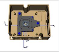
CAD construction of modified titanium fle.X-Plate in a case housing a detector in its central hole.
