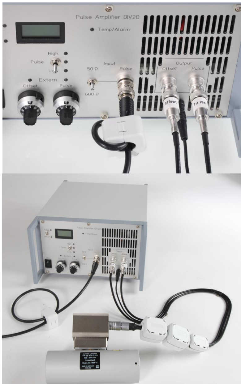
Fig. 4: Connecting the Modulator-cable to the DIV 20 and ferrite to Pulse-Input
